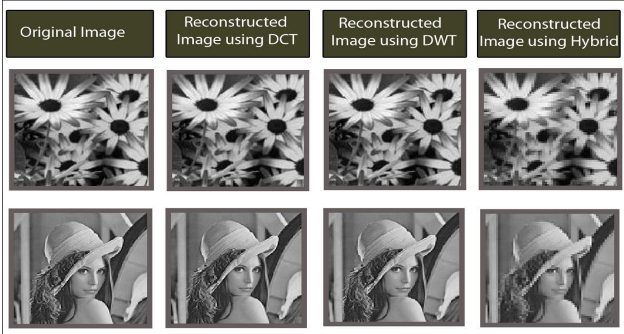
Fig9. Reconstructed Image using DCT,DWT,HYBRID(DCT-DWT)
